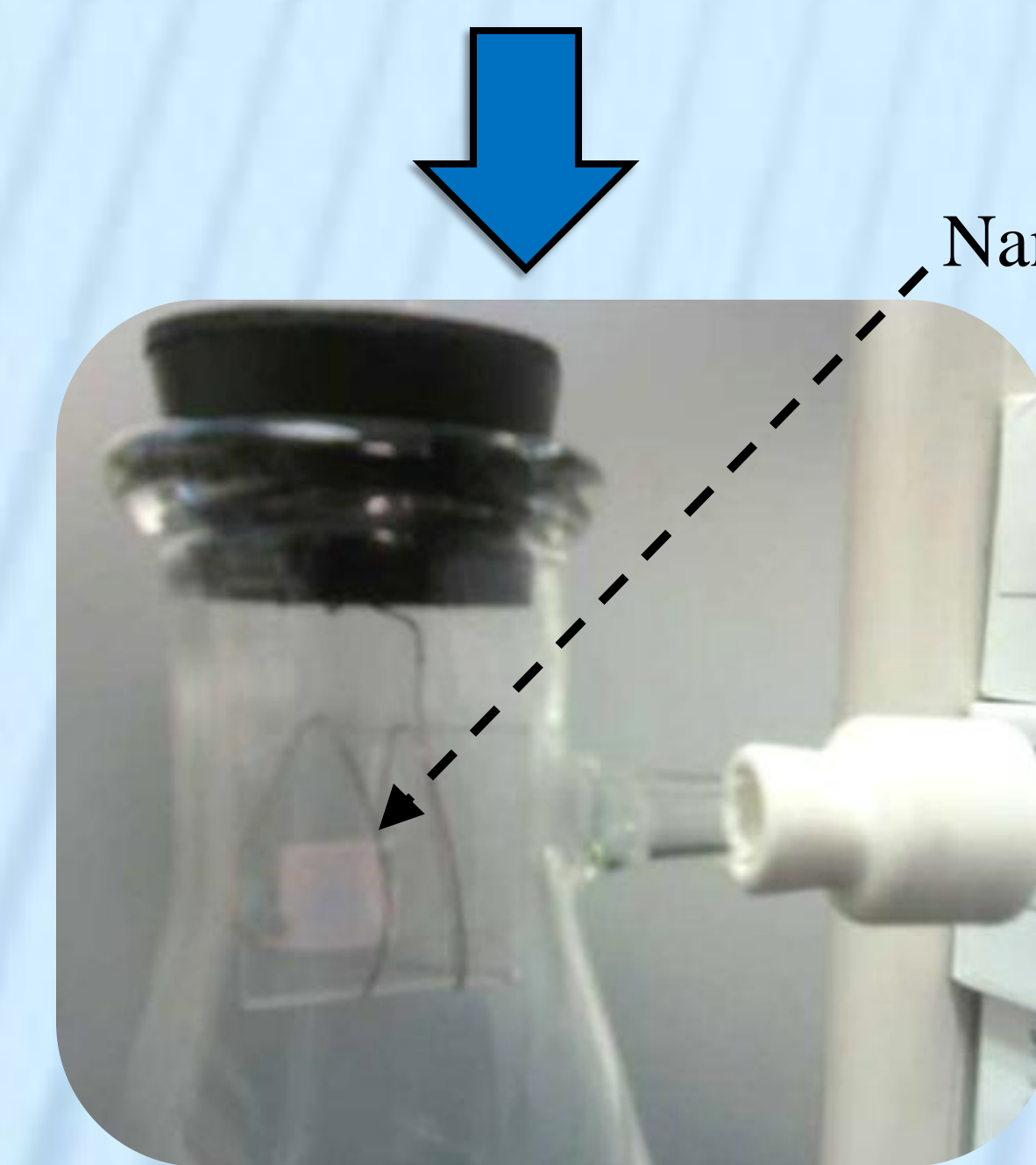
Figure 2 – 1 cm 2 nanospring mat on ITO electrode and glass.
